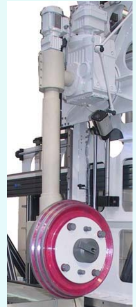
Grinding wheel mounted to swivelling and rotation unit.
