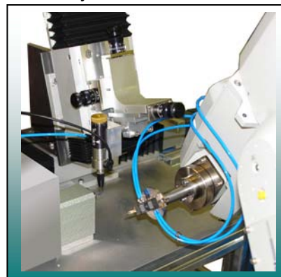
Basic varnishing unit with 6-axes bent-arm robot
