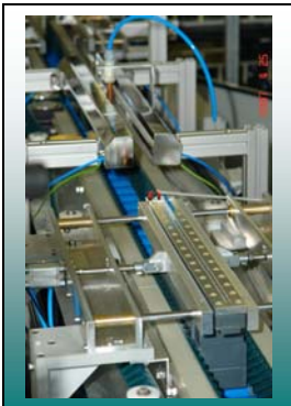
Loading of fixtures and drying unit
