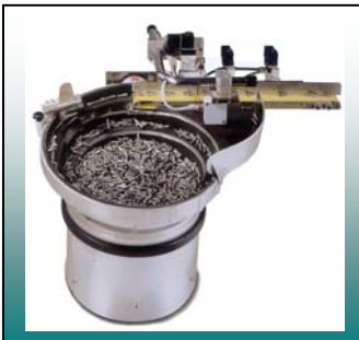
Precision bowl feeder for bulk material
